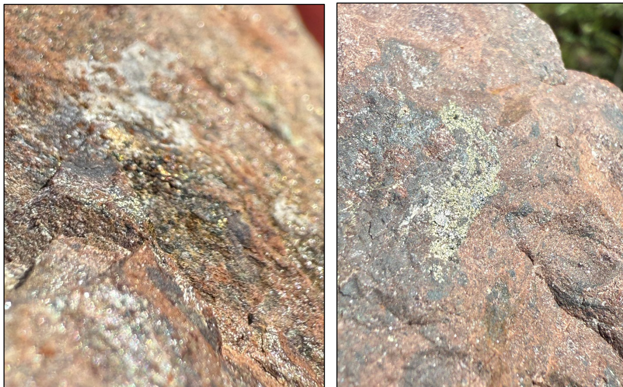
Figure 3 (Left and right): Example of the disseminated chalcopyrite mineralisation identified in rock samples collected for uranium testing at the Queens Gift Uranium prospect.
