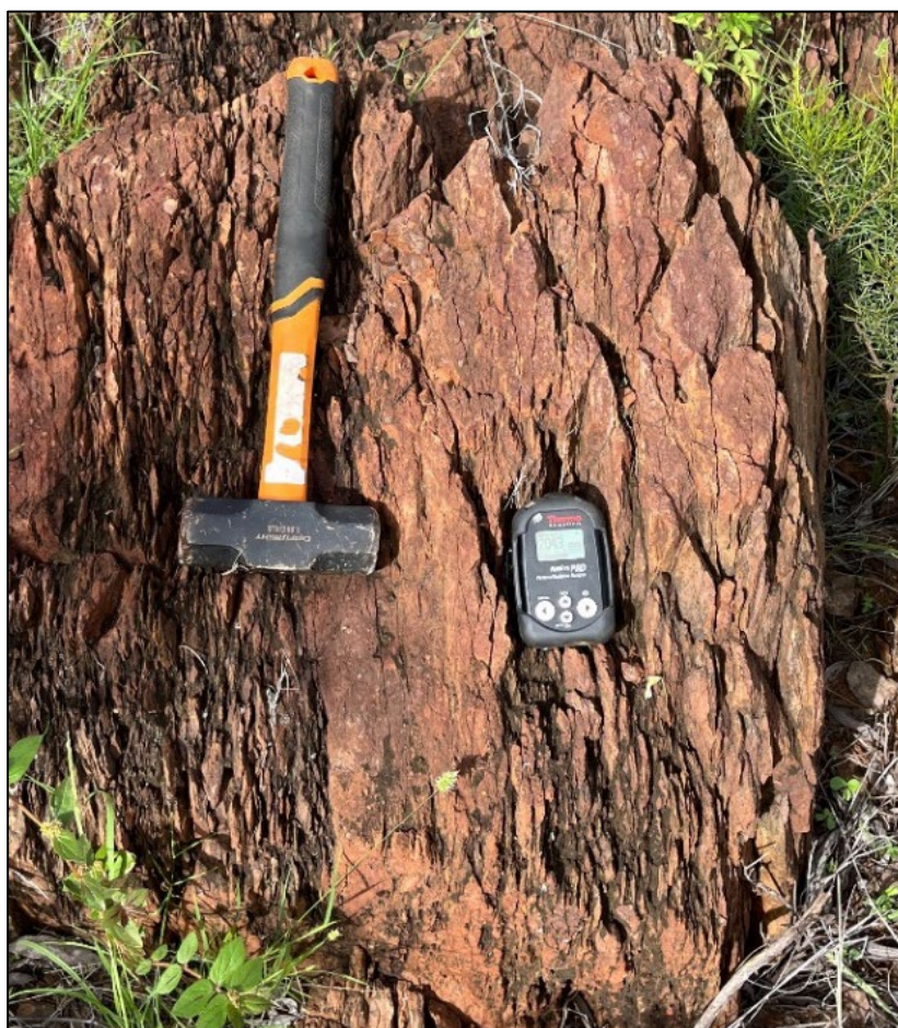
Figure 2. ASR0023 – outcrop showing sheared hematite and albite altered basalt with RadEye scintillometer.
