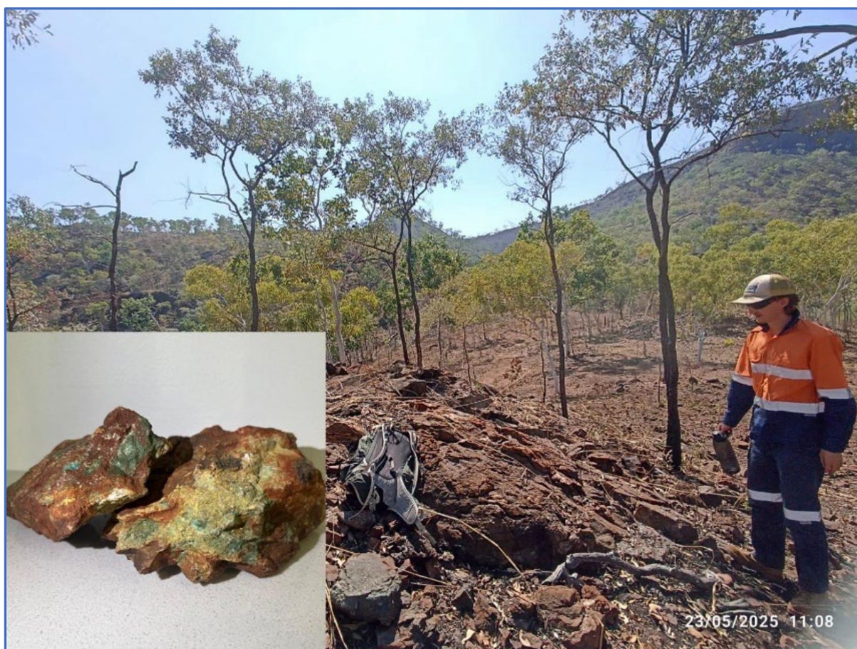
Figure 1. Outcrop sampling at Speewah Nth. Inset gossanous malachite sample with antimony.
