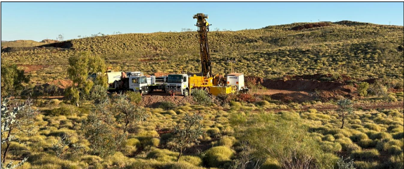
Figure 1: Diamond drill rig undertaking metallurgical and geotechnical drilling at the Tabba Tabba Project
