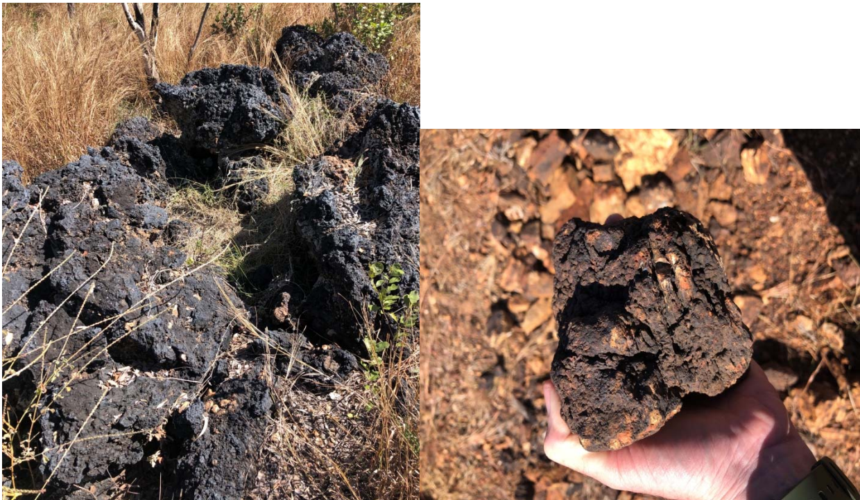
Figure 7 (above) left Massive Mn ore (Psilomelane) at Masterton 2 workings and Mn sample from the Quarry Prospect.
